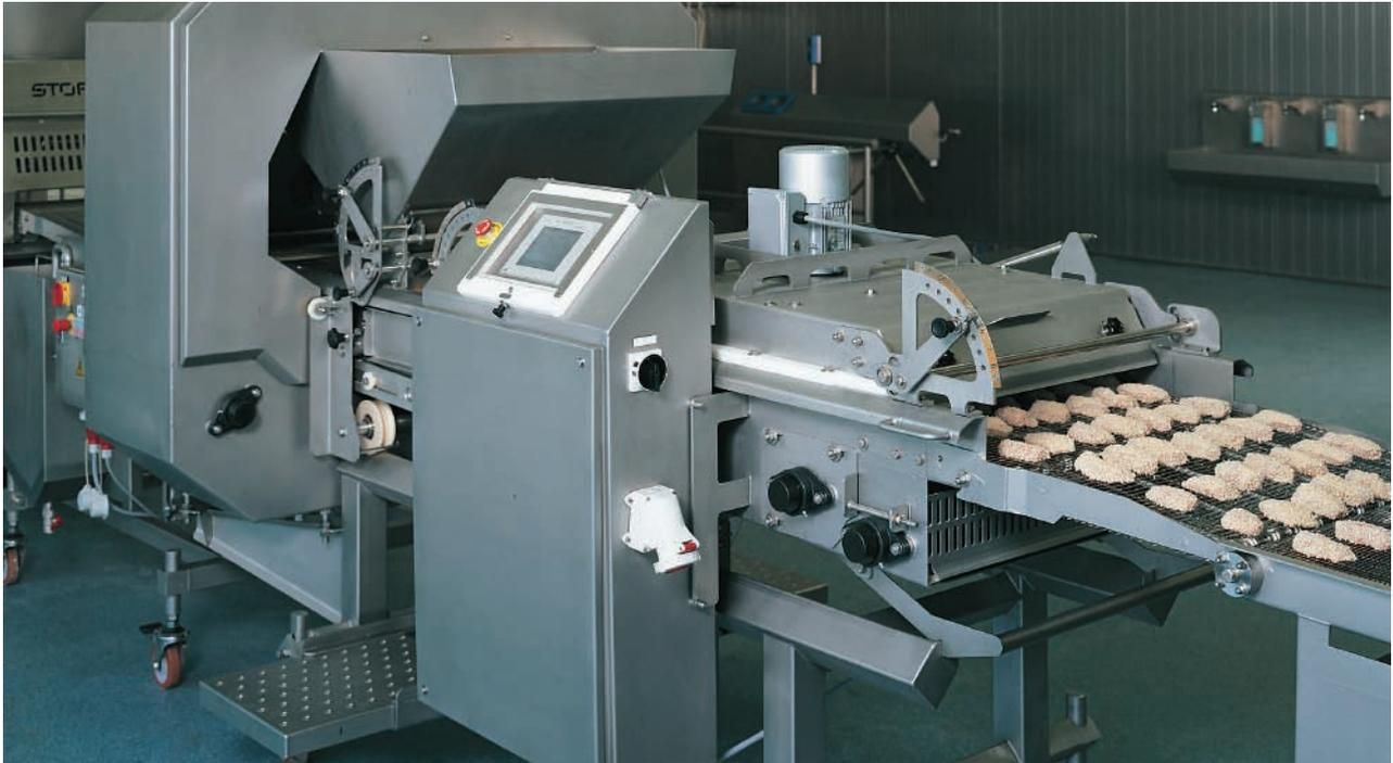
With RotoCrumb the grinding and separation of crumb is a thing of the past. Townsend Further Processing has replaced the traditional screw conveyor with a revolutionary new transport mechanism. What is more, a comprehensive dosing system ensures that only a minimum volume of crumb is in circulation at any one time. This allows standard crumb, mixtures of crumb and delicate ingredients such as Japanese crumb to be handled.
