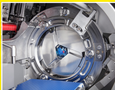
The iris separator ensures clean sausage ends and careful portioning.
