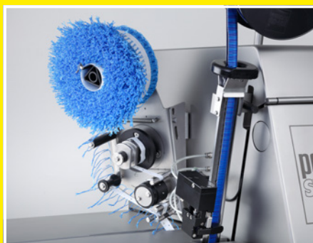
The iris separator ensures clean sausage ends and careful portioning.
