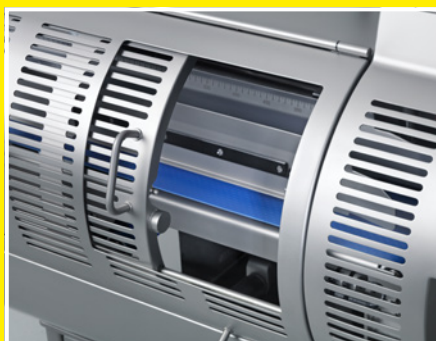
The overspread ensures the air-free loose filling of moulded products.
