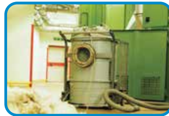
Mobile vacuum cleaner Air-volume: 230 m 3 /h Vacuum: 200 mbar Relative suction performance: 23% Filter capacity: 70 lt
