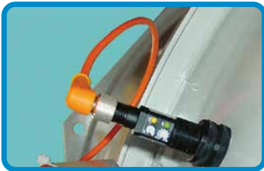
Level control device (optical): signal for a variety of displays or control commands
