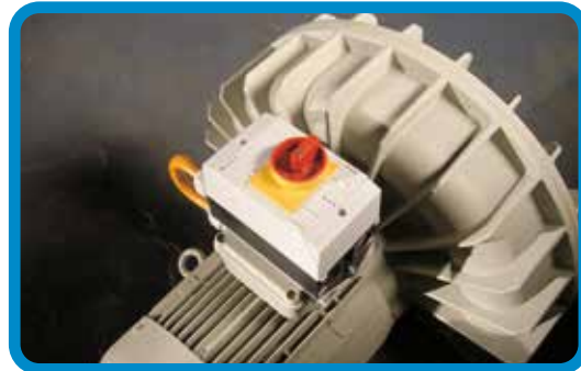
Electrical motor switch with fuse control attached to motor
